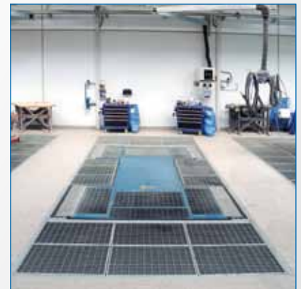
Flush mounted with low pit depth.
