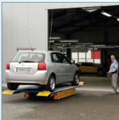
The cars are on lifts from the moment the work is started right through to the final inspections. It can safely and quickly be moved to subsequent workstations.
