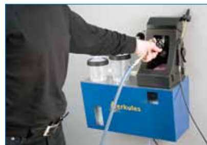
Rinse the paint channel
