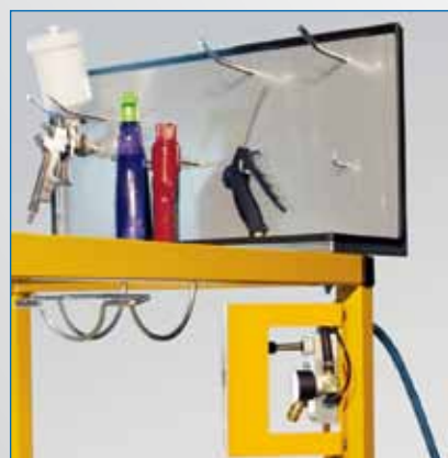
On the platform are several air supplies as well as storage space for the tools. Therefore they are always within reach.
